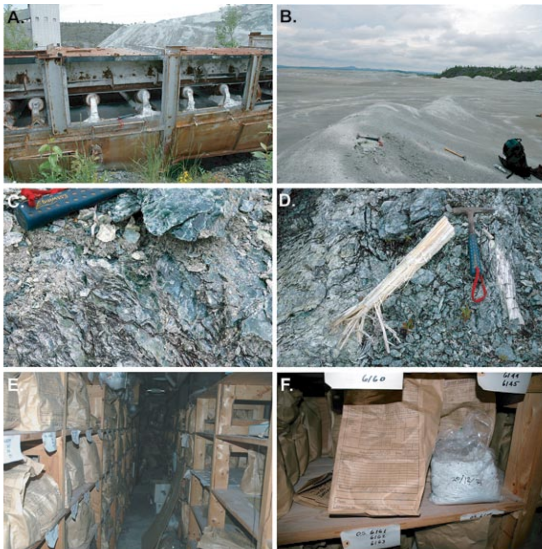
FIG. 3. Photographs of some of the locations of the collected samples. A) Sample #3 was collected from this conveyor belt next to the rock pick. The belt was located next to the old mill and is assumed to be carrying this material to the tailings piles. B) Sample #6 was collected from the top of this tailings pile (in front of the rock pick), which is located on the south side of pit C. C) Sample #7, an in-place sample showing “fish-scale” morphology, was taken from the footwall on the north side of pit C. D) This photo shows sample #9, which was dug out of the western end of the Pennington dyke from pit C. Also shown is an in-place sample (to the right of the rock pick). E) All six samples labeled #10 came from this storage area in the basement of the laboratory building. F) This photo shows a close-up of one of the plastic bags containing processed chrysotile, stored in paper bags seen in Figure 3E. This is sample #10b3, collected at the mine on December 20, 1979.
